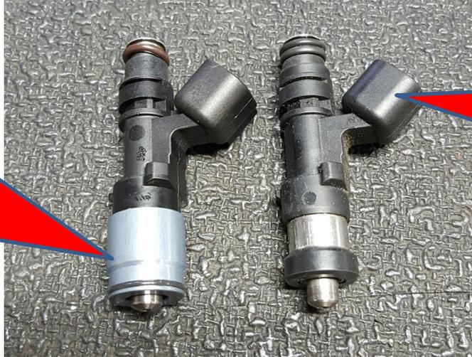
Picture shows the New Injector Dynamics top feed injector body (left) versus the old ID injector body (right).
