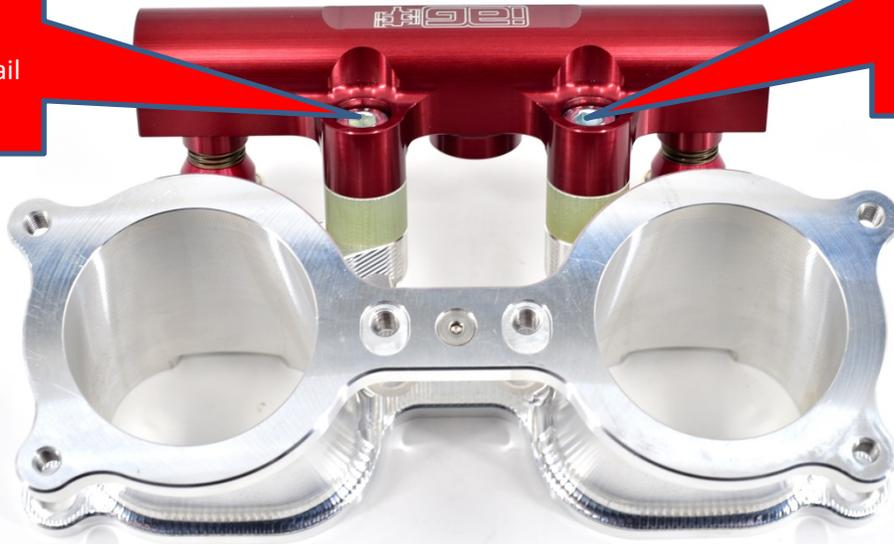
6. Shows IAG Fuel Rail to TGV mounting points with (x2) large phenolic fuel rail spacers. Also illustrates Injector Dynamic injector fitment.
