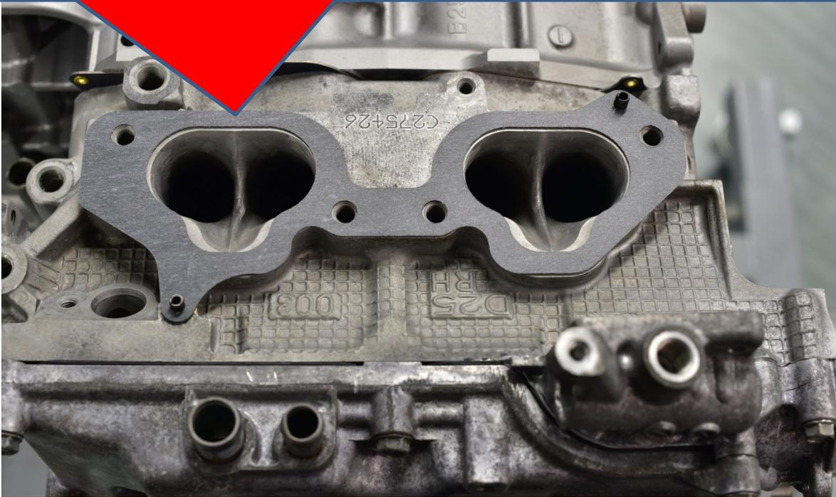
3. Next, carefully place each TGV on the cylinder head. Use (x8) of the included M8x25 hex head bolts to secure the each TGV on to your engine as shown below. Torque the bolts to 18.4 ft/lbs.
