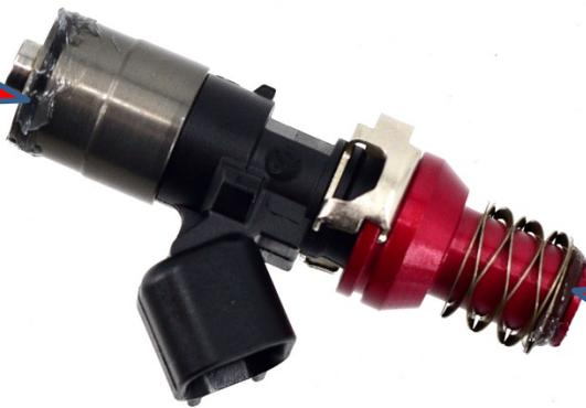
Apply a thin layer of o-ring lube around the upper injector adapter o-ring for each injector. This helps protect the o-ring from damage during install.
