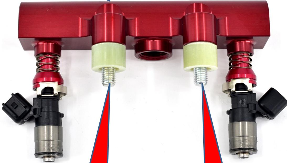
M8x30 Socket head bolt place through the fuel rail with large phenolic spacer shown
